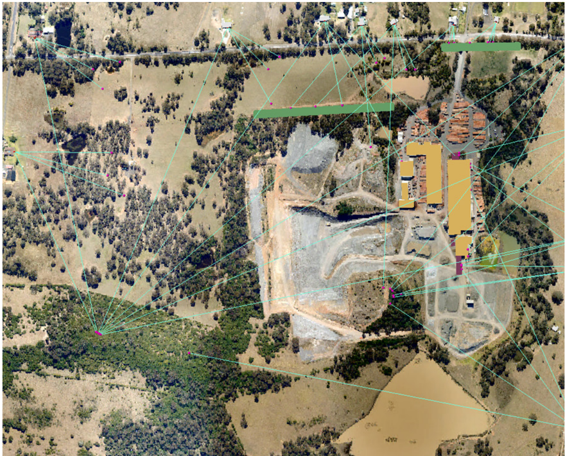
Figure 7-40 Output from ArcScene identifying targets and lines of sight to the project site
